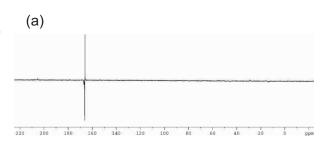
By the application of a taylored pulse sequence, it is possible to obtain an in-phase signal
