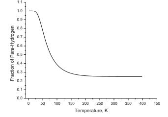
Normal hydrogen molecule H<sub>2</sub> consists of 75% ortho- and 25% para-hydrogen.
