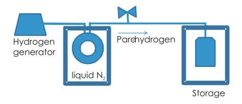
Higher level of para-H<sub>2</sub> can be attained by using a cryo-system, operating at temperature lower than 77 K.
