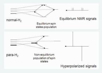
In order to transform the antiphase polarization into an in-phase signal, an appropriate pulse sequence can be applied into a very low field NMR spectrometer.
